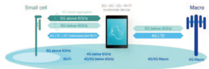
Fig. 3. The 5G multiconnectivity concept. Source: www.qualcomm.com
