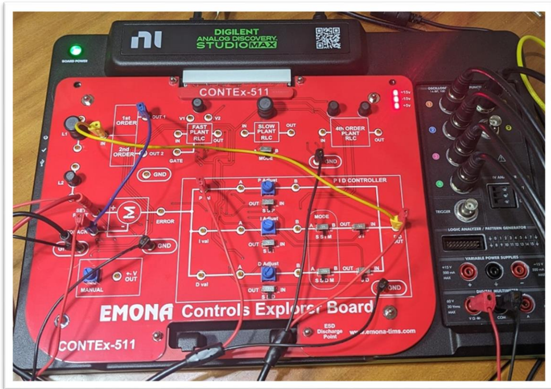
Figure 69: Patching for PID loop with underdamped plant
