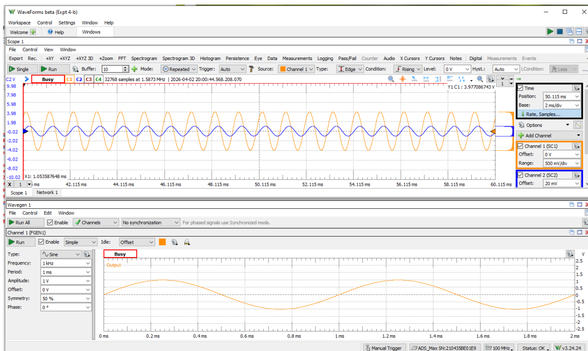
Figure 14: Sample WAVEFORMS instrument panel from a workspace file
