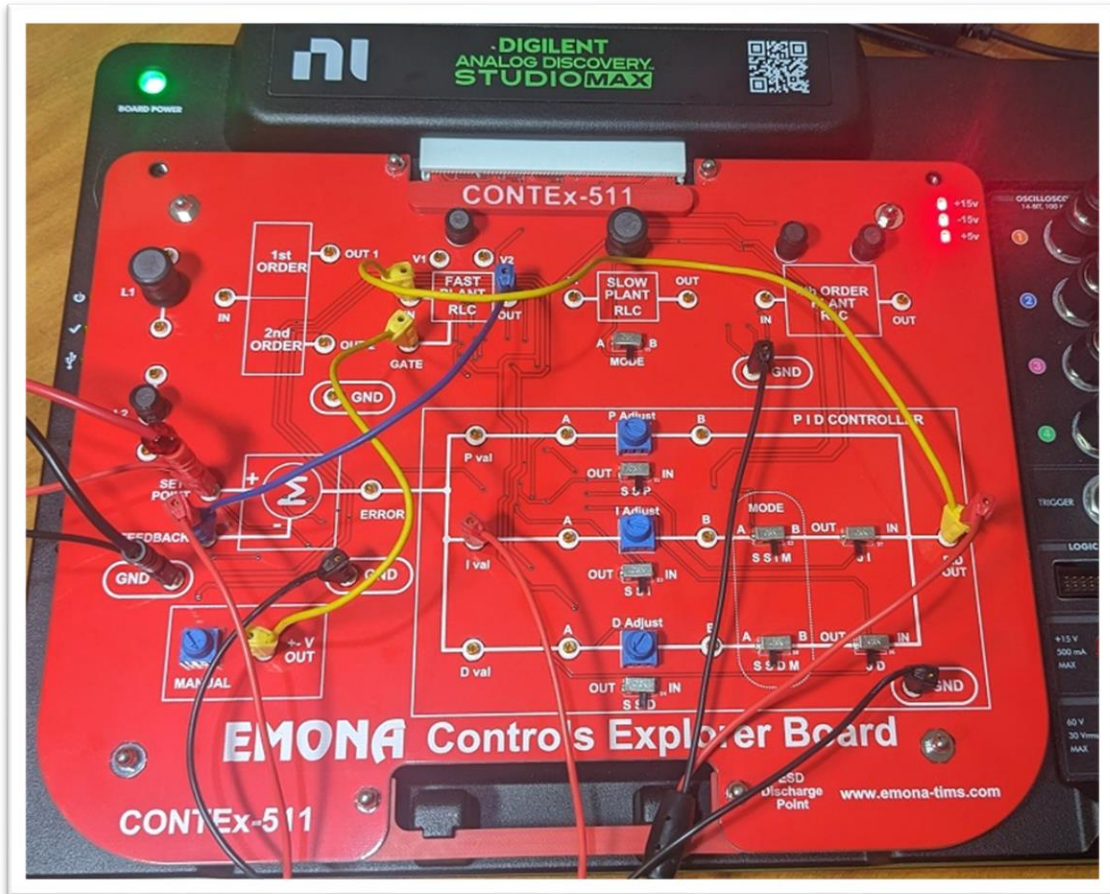
Figure 75: Patching for PID loop with underdamped plant
