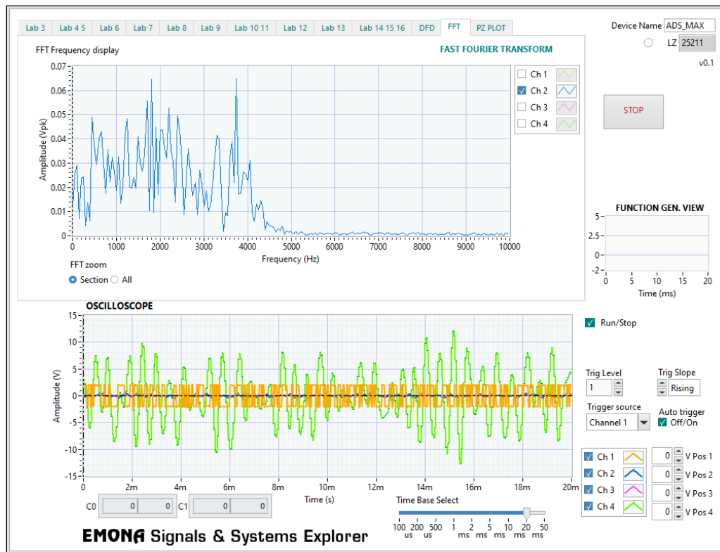
Figure 15: FFT display used to view experiment setup with flat noise spectrum as input signal
